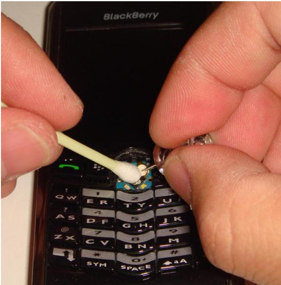
When you clean the peeled off part, make sure you're not swabbing the sticky section or you'll have to figure out how to make this stick back in the phone.
