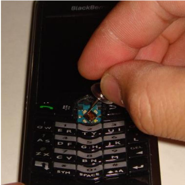
You can now put the trackball back in (making sure that the two pegs are lined up horizontally) and then put the ring back on.
